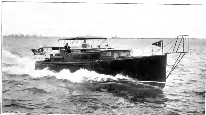
This serviceable type of cruiser, fitted for fishing, is becoming very popular on Gulf, Atlantic, and Pacific Coasts. The Marline is 51'6" by 12'6" by 2'10". She was designed by Eldredge & McInnis, Inc., and built by Fred D. Lacey, Inc. Her two Sterling Dolphin 6-cylinder engines give her a speed of 28 miles an hour.
